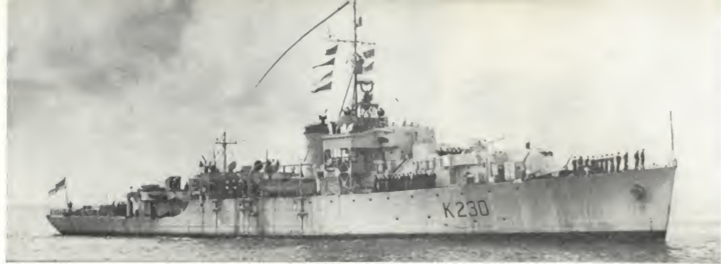
HMS Wear entering Portsmouth to pay-off in August 1946. She has a typical close armament of seven single 20 mm Oerlikons, in addition to her two single 4 inch (Wright & Logan).
